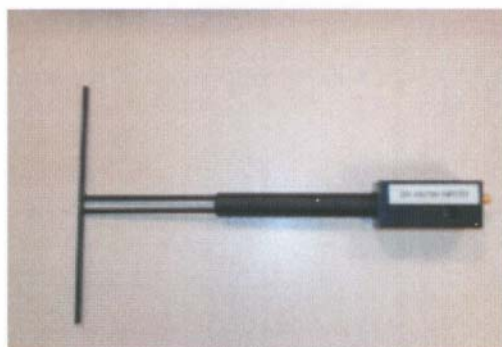
Figure 1 – Satimo COMOSAR Validation Dipole
