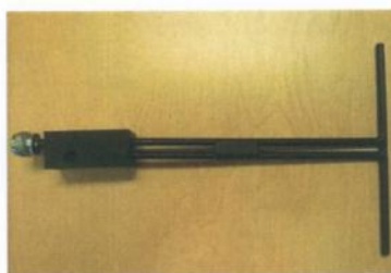
Figure 1 – MVG COMOSAR Validation Dipole
