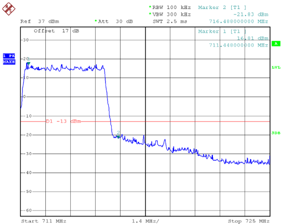
Higher Band Edge Plot for QPSK -RB Size 75, RB Offset 0
