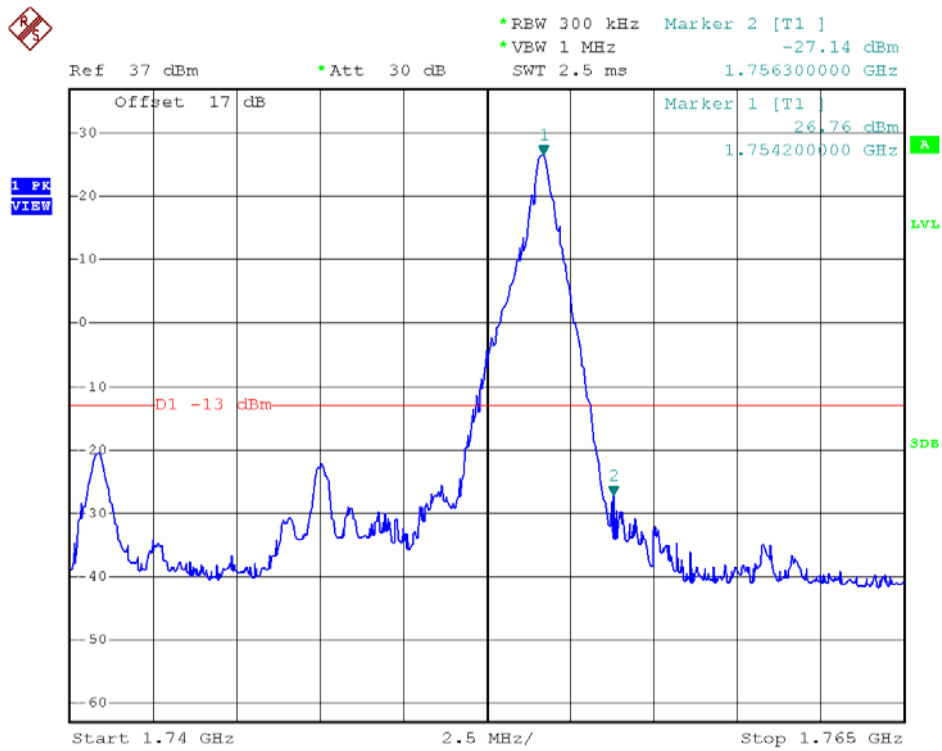
Higher Band Edge Plot for QPSK-RB Size 1, RB Offset 74
