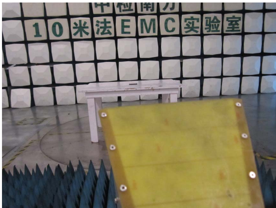
Radiated emission-above 1GHz
