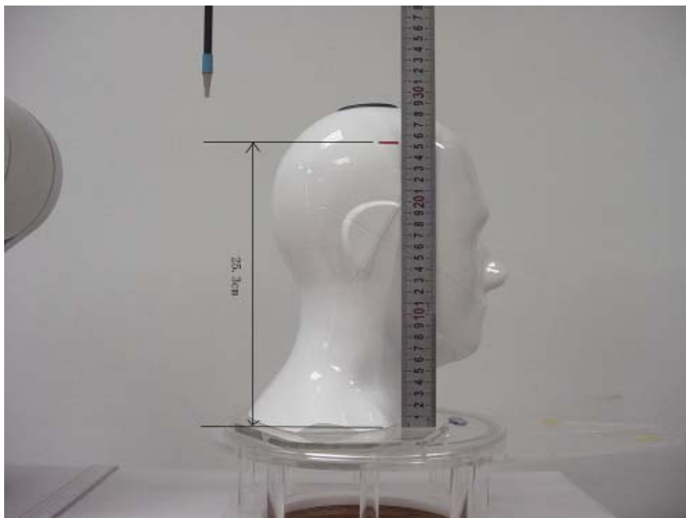
Fig.2 The depth of head tissue in SAM
