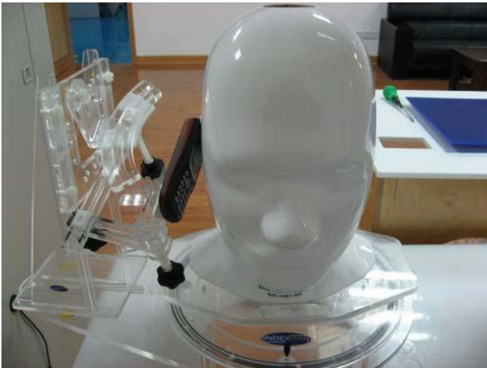
Fig.6 EUT Right Head Tilt15 Position
