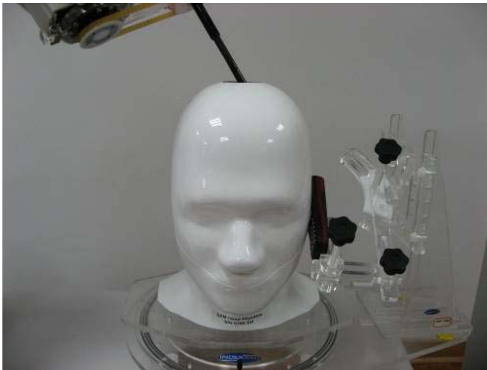
Fig.3 EUT Left Head Touch Cheek Position
