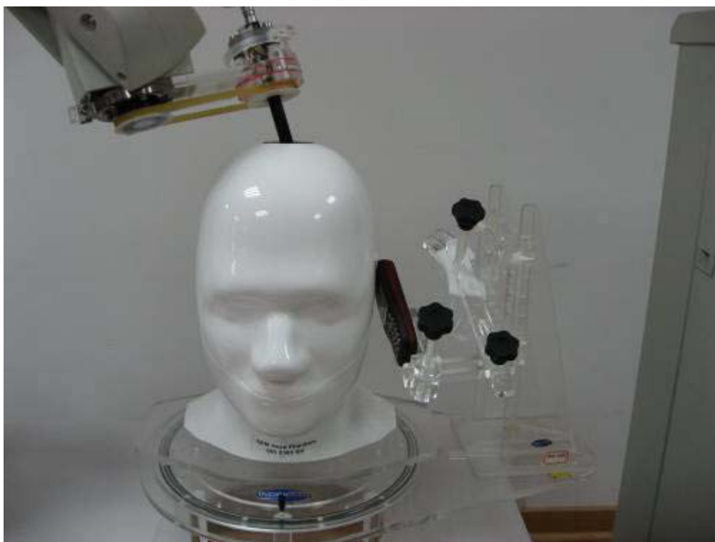
Fig.4 EUT Left Head Tilt15 Position
