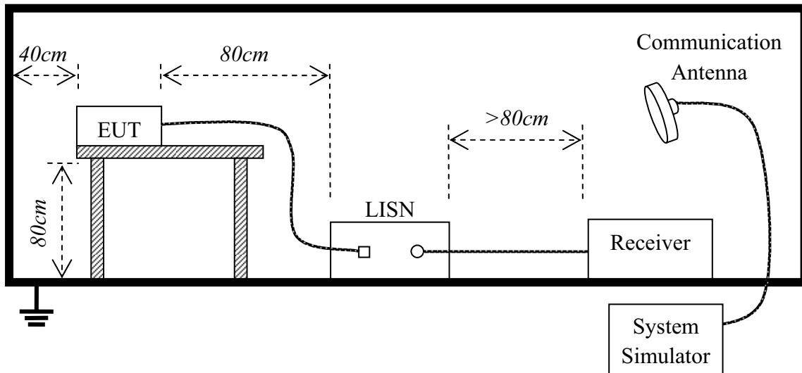
1. The test is performed in a Shield Room; the factors of the test system are calibrated to correct the reading.
