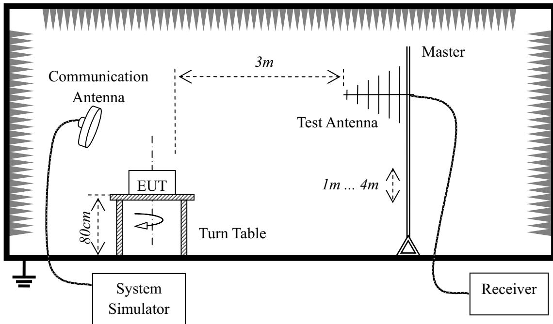
1. The test is performed in a Semi-anechoic Chamber; the factors of the test system are calibrated to correct the reading.
