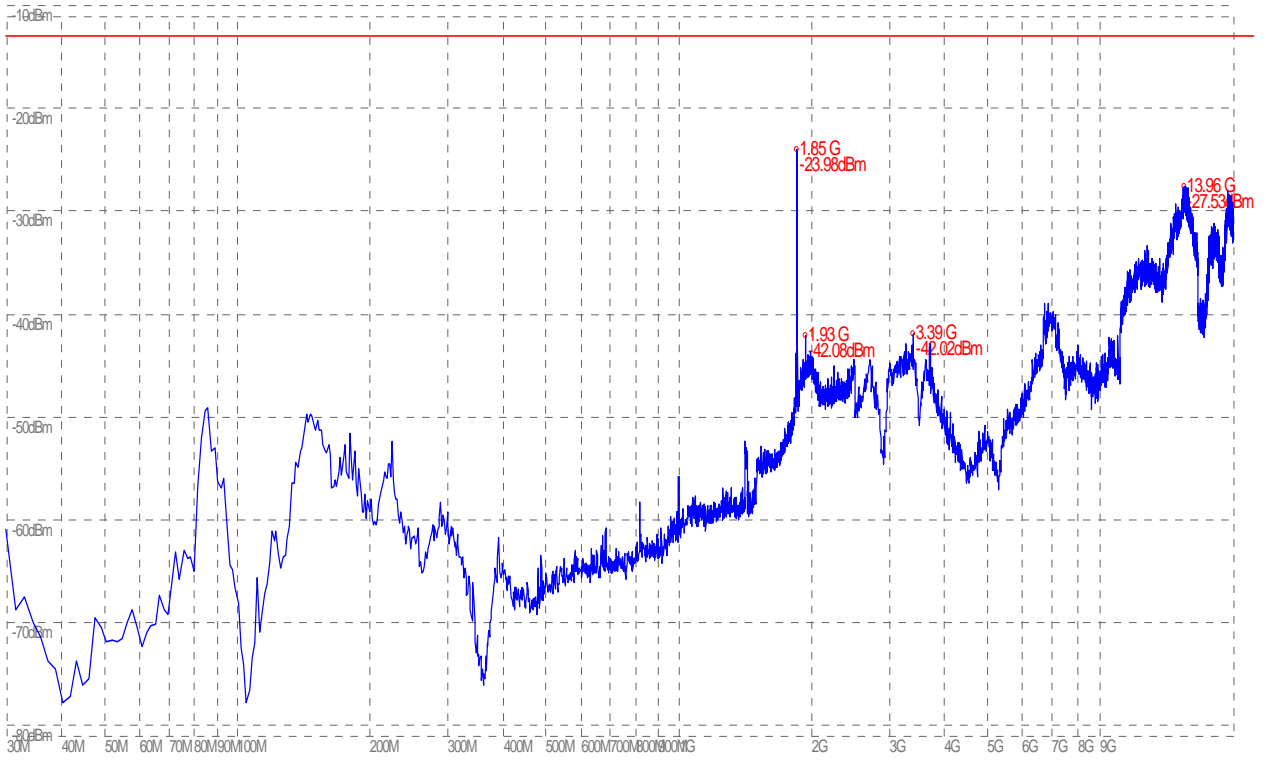
(Plot J.1: HSUPA 1900 MHz Channel = 9262, Test Antenna Horizontal)
