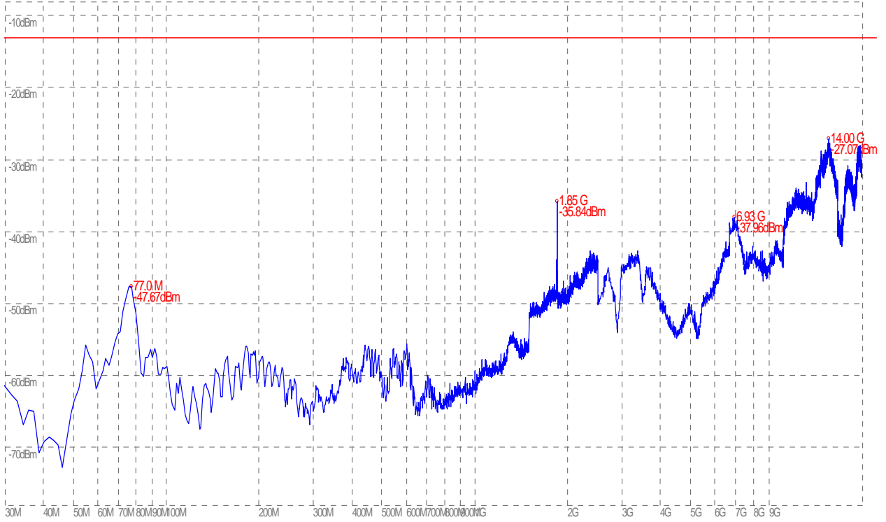
(Plot F.1: WCDMA 1900MHz Channel = 9262, Test Antenna Horizontal)
