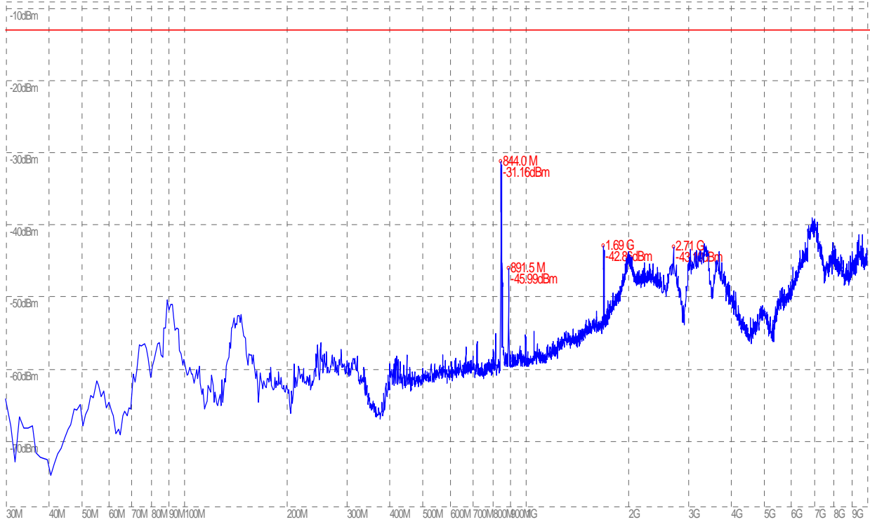
(Plot I.5: HSUPA 850MHz Channel = 4233, Test Antenna Horizontal)
