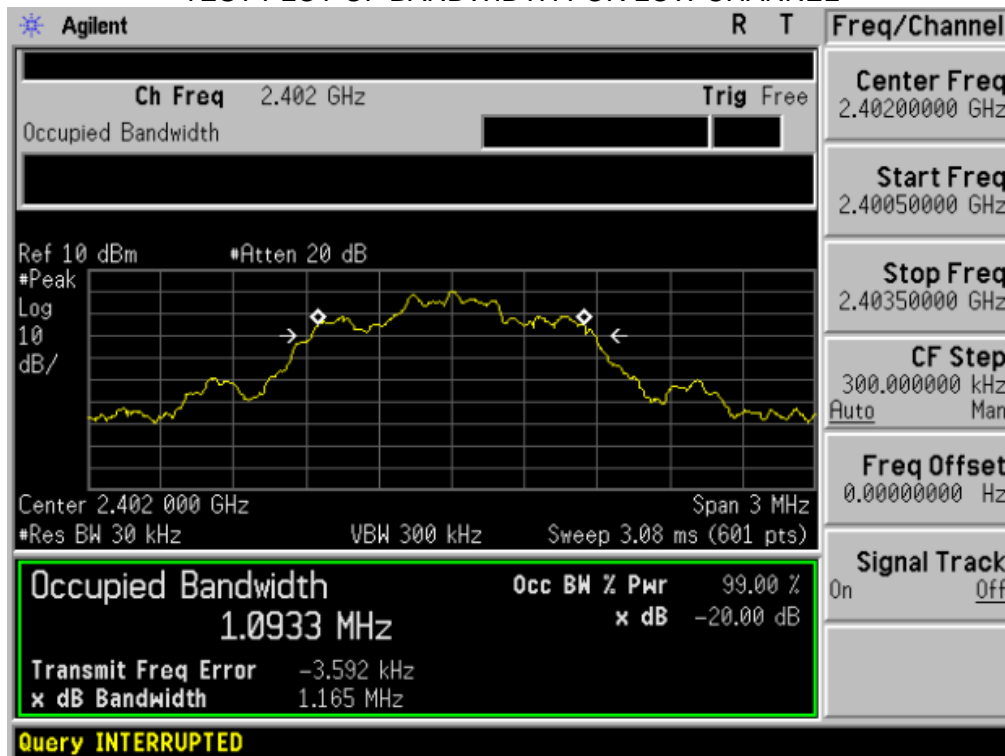
TEST PLOT OF BANDWIDTH FOR LOW CHANNEL
