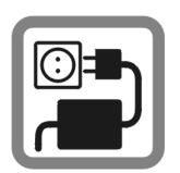
The mains voltage (V) specified on the power supply unit must not be exceeded. Otherwise the charging device may be damaged.
