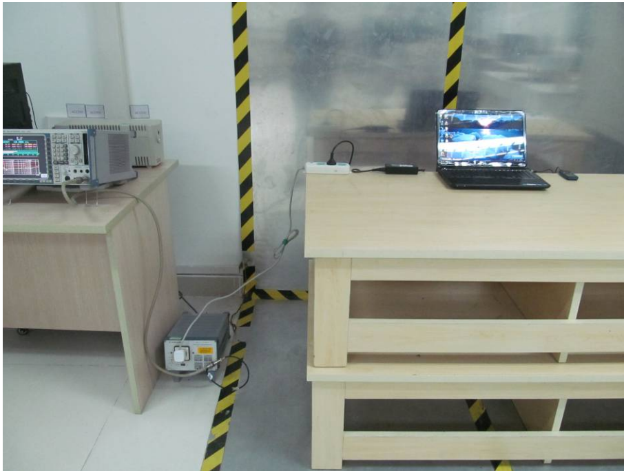
FCC RADIATED EMISSION TEST SETUP
