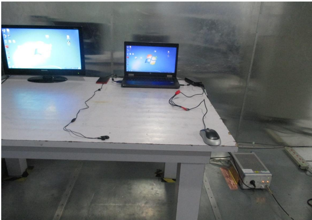
Conducted Emission Test setup photos
