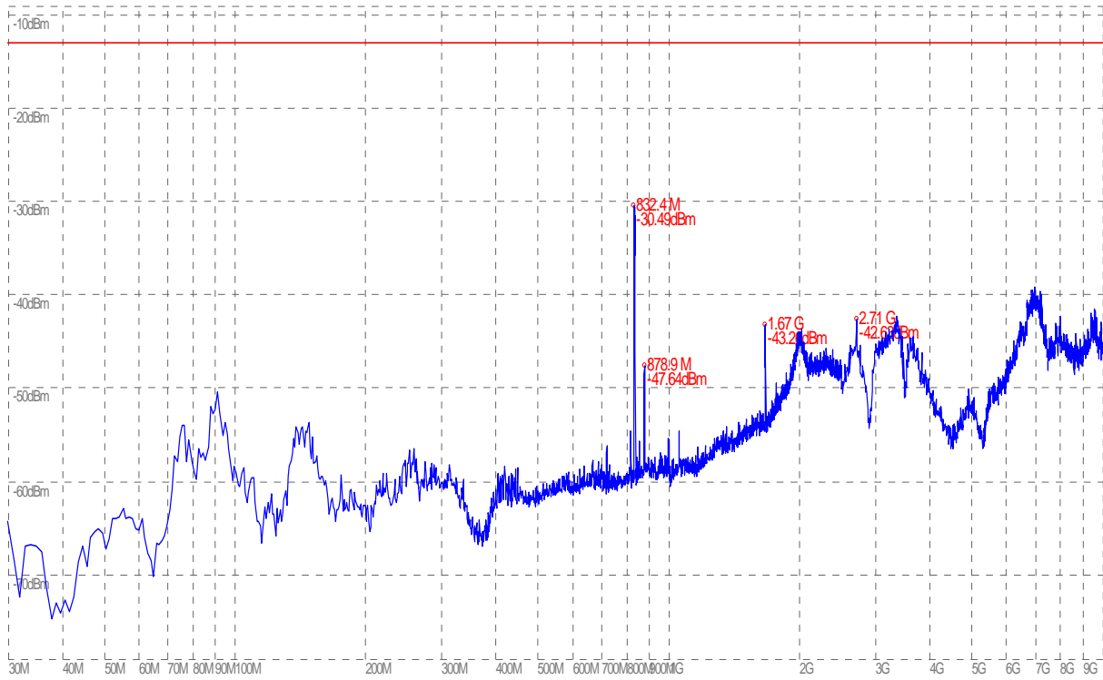
(Plot G.5: HSDPA 850MHz Channel = 4233, Test Antenna Horizontal)
