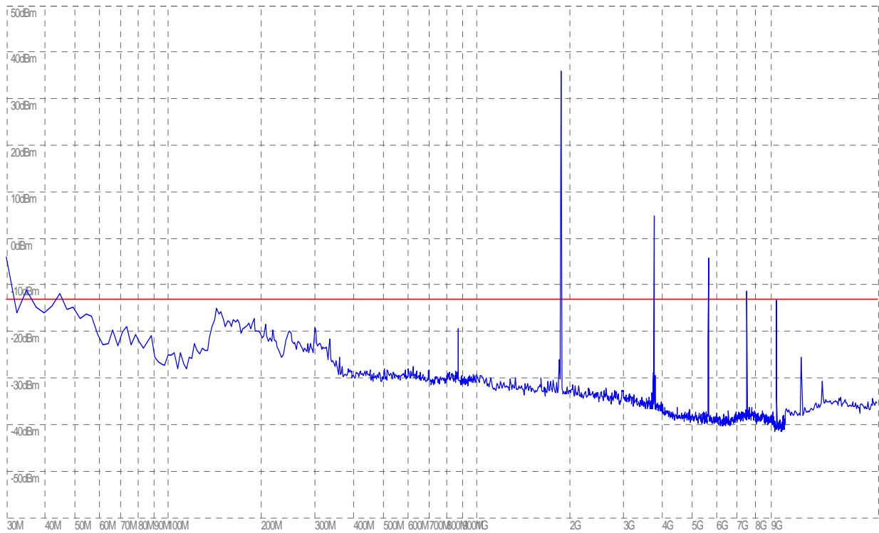
(Plot D4 : EGPRS 1900MHz Channel = 661, Test Antenna Vertical)
