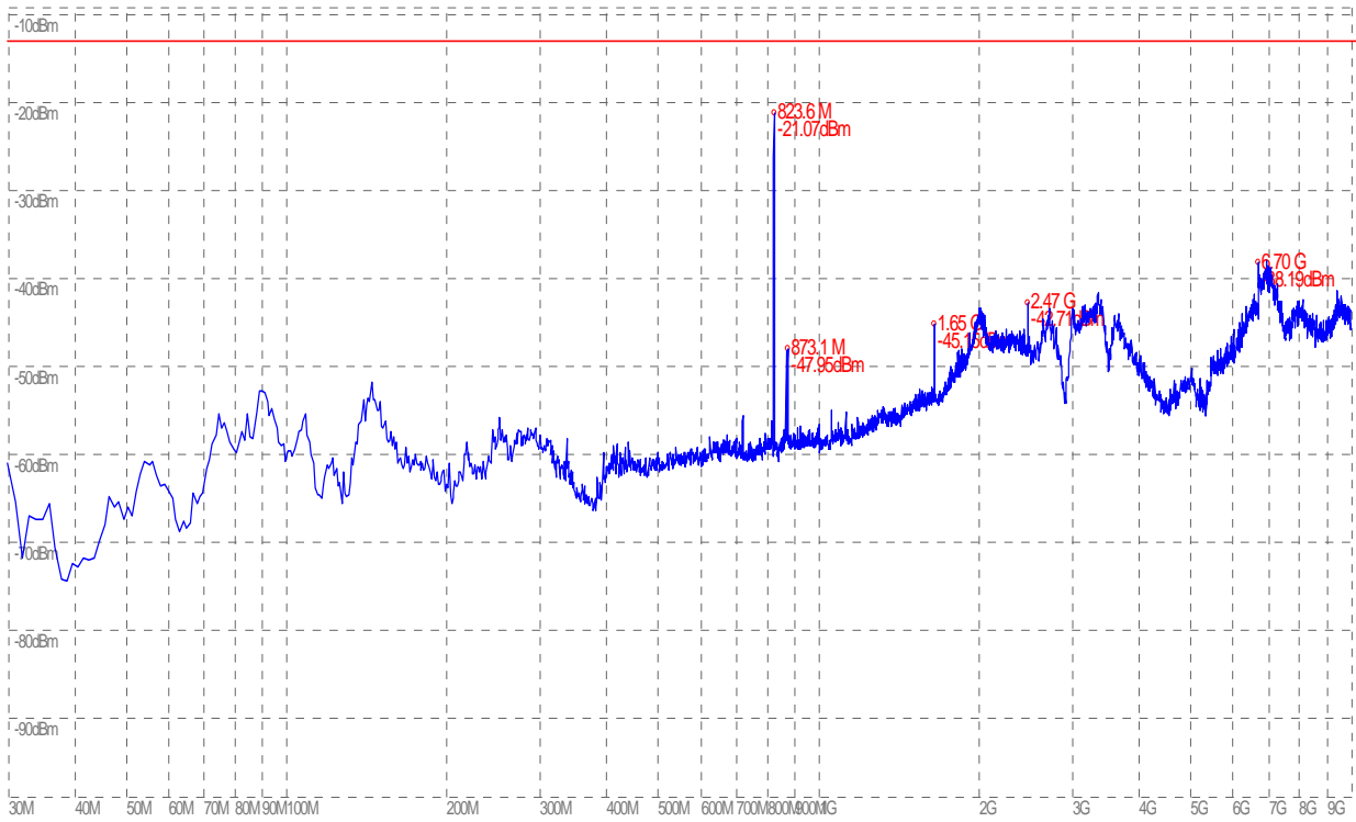
(Plot C1 : EGPRS 850MHz Channel = 128, Test Antenna Horizontal)
