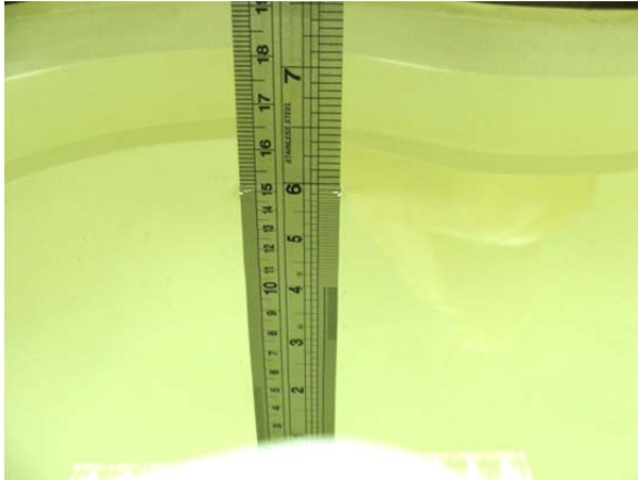
Fig 6.1 Photo of Liquid Height for Head SAR
