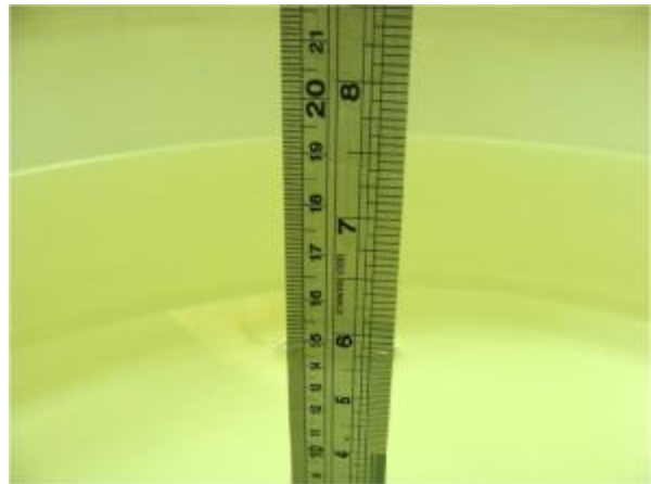
Fig 6.2 Photo of Liquid Height for Body SAR
