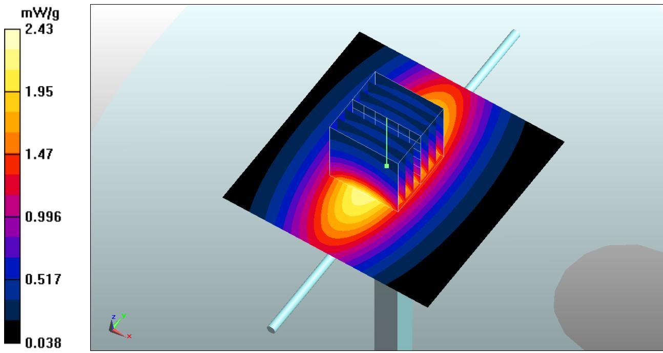
**System Check\_Body\_835MHz\_110318****DUT: Dipole 835 MHz**
