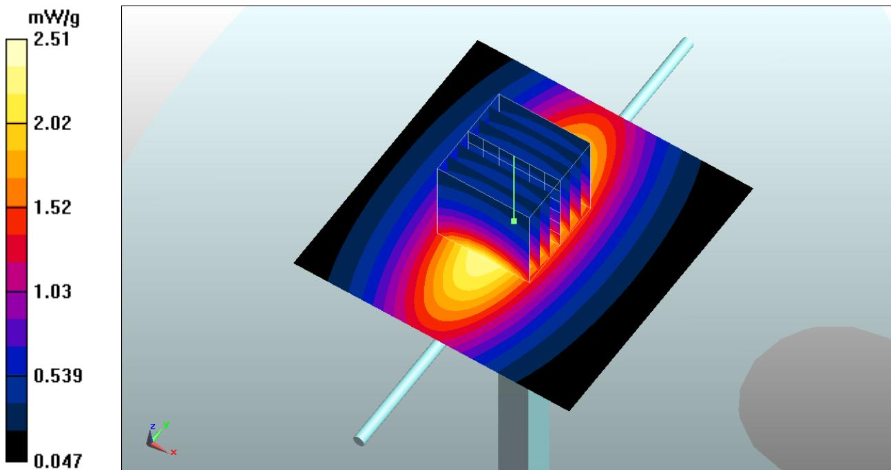
**System Check\_Head\_1900MHz\_110318****DUT: Dipole 1900 MHz**
