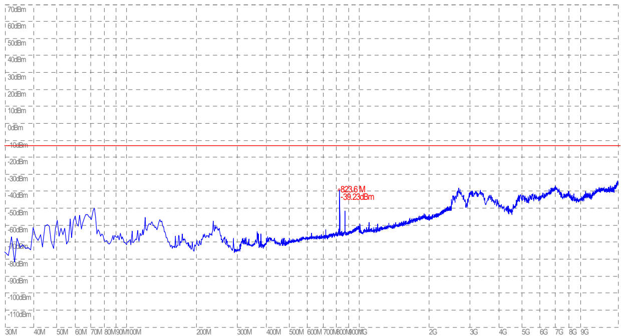
(Plot A.2: CDMA 800MHz Channel = 1013, Test Antenna Vertical)
