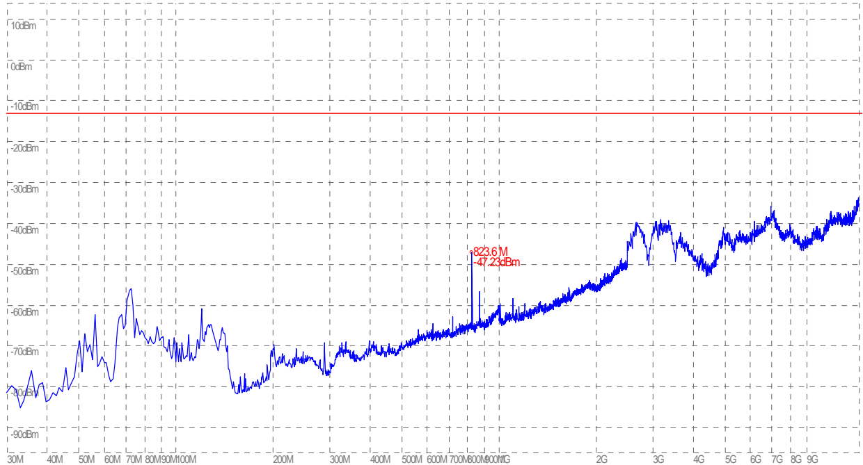
(Plot A.1: CDMA 800MHz Channel = 1013, Test Antenna Horizontal)
