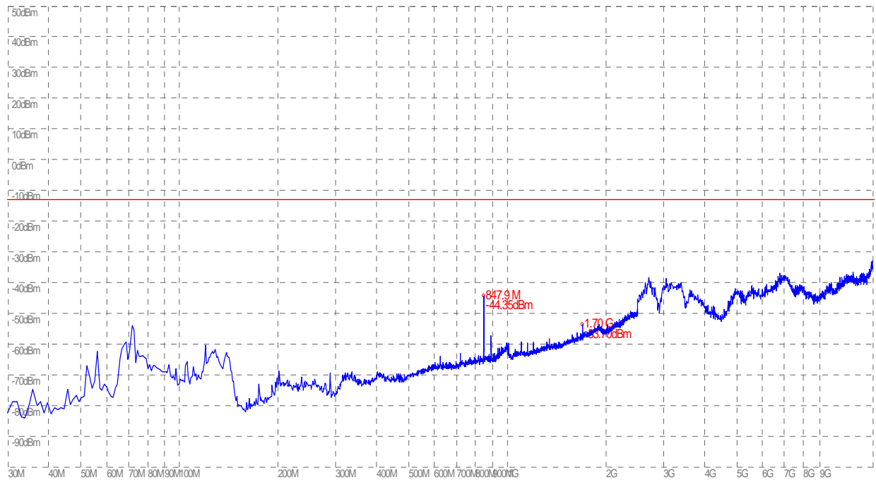
(Plot C.1: CDMA 800MHz Channel = 777, Test Antenna Horizontal)
