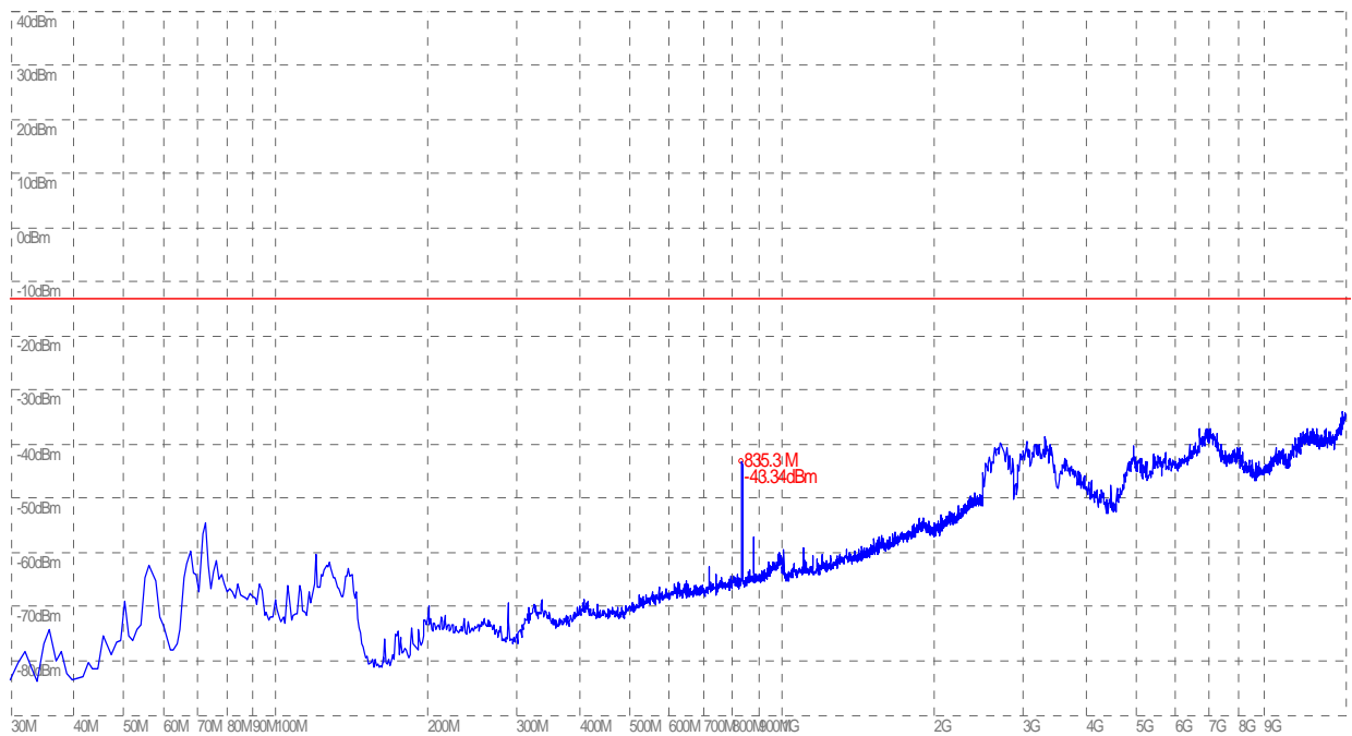
(Plot B.1: CDMA 800MHz Channel = 384, Test Antenna Horizontal)
