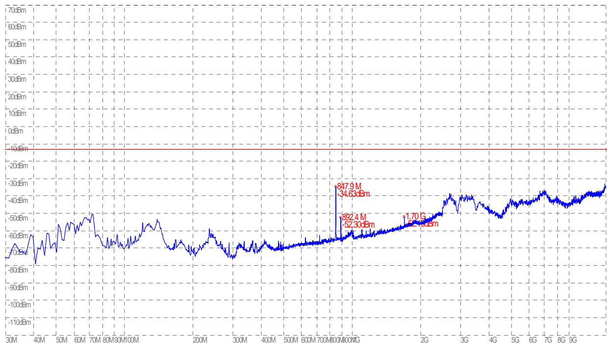
(Plot C.2: CDMA 800MHz Channel = 777, Test Antenna Vertical)
