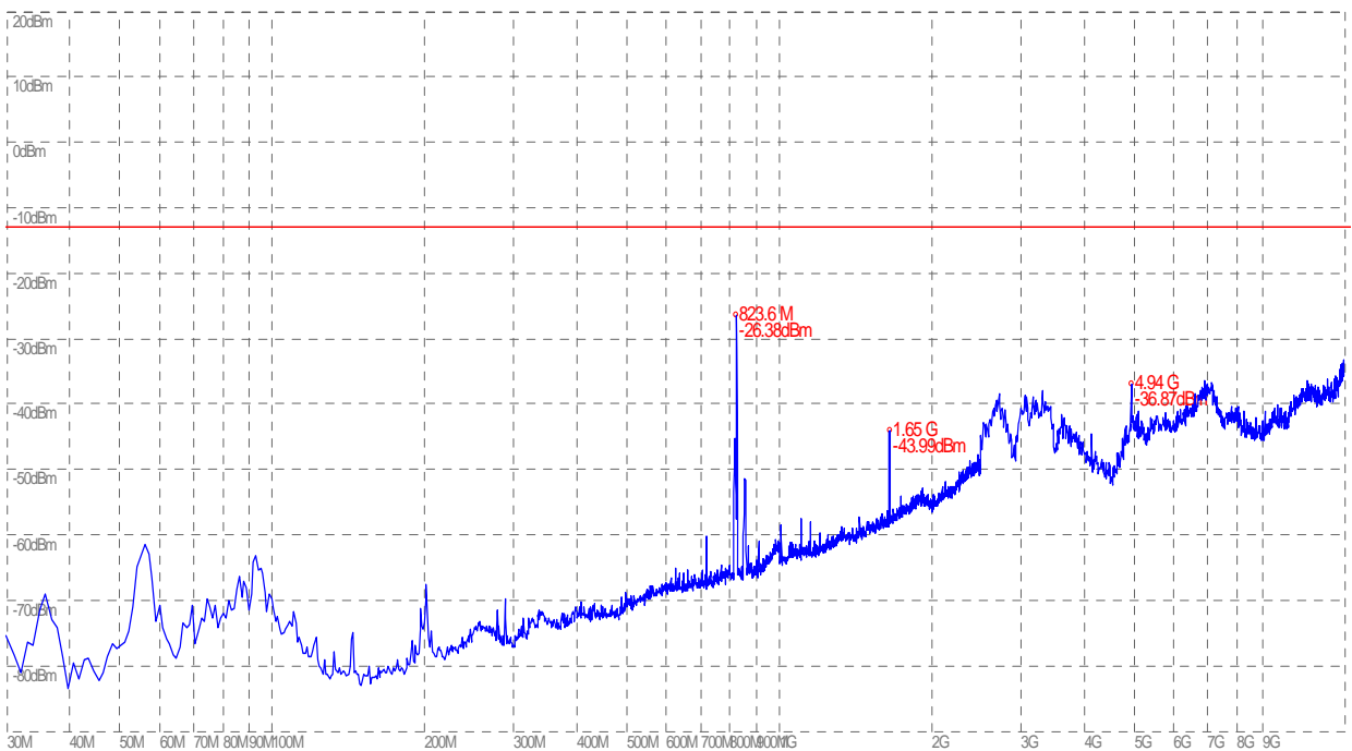
(Plot A.2: Plot when the TCH number set to 1013, Test Antenna Vertical)
