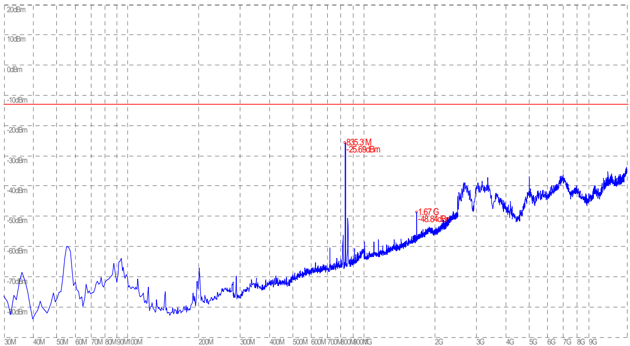
(Plot B.2: Plot when the TCH number set to 384, Test Antenna Vertical)
