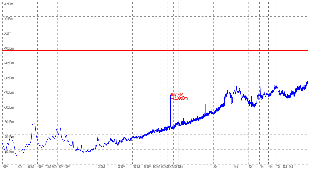
(Plot C.1: Plot when the TCH number set to 777, Test Antenna Horizontal)
