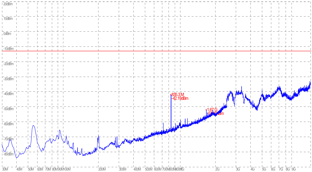
(Plot B.1: Plot when the TCH number set to 384, Test Antenna Horizontal)
