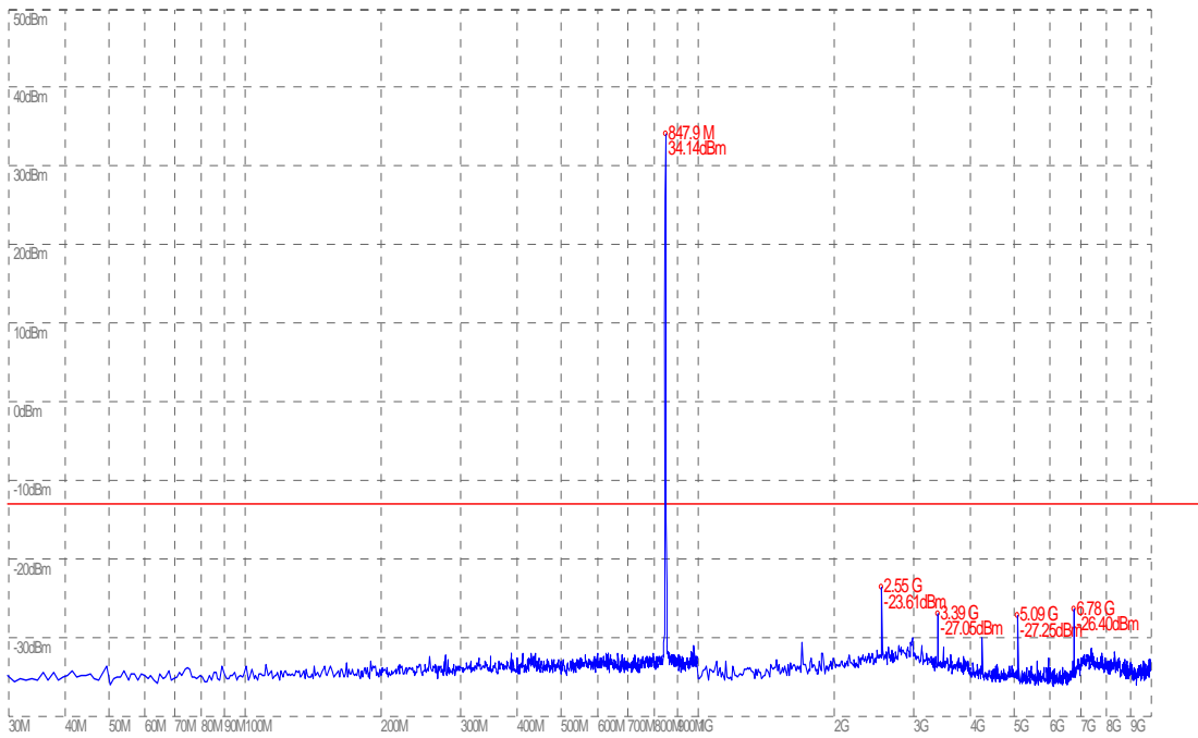
(Plot C: GSM 850MHz Channel = 251, 30MHz to 9GHz)
