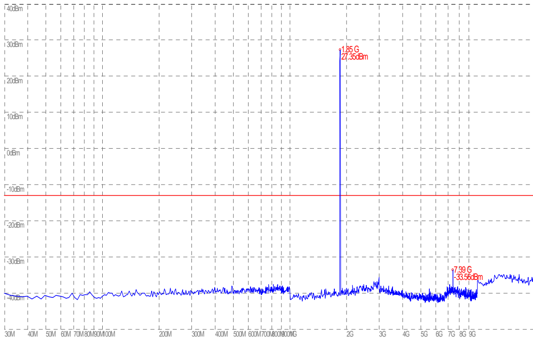
(Plot D: GSM 1900MHz Channel = 512, 30MHz to 20GHz)
