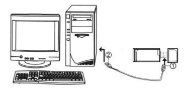
After data card inserted, in the down right corner of the computer screen, there will be a hint that "Fond new hardware". In the process of installation there will be the following hint, please select "Continue Anyway".
