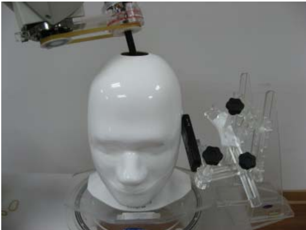
Fig.4 EUT Left Head Tilt15 Position
