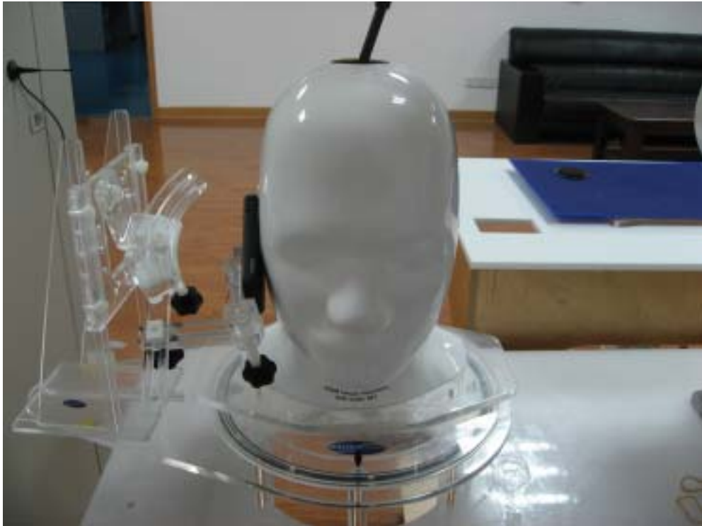
Fig.5 EUT Right Head Touch Cheek Position
