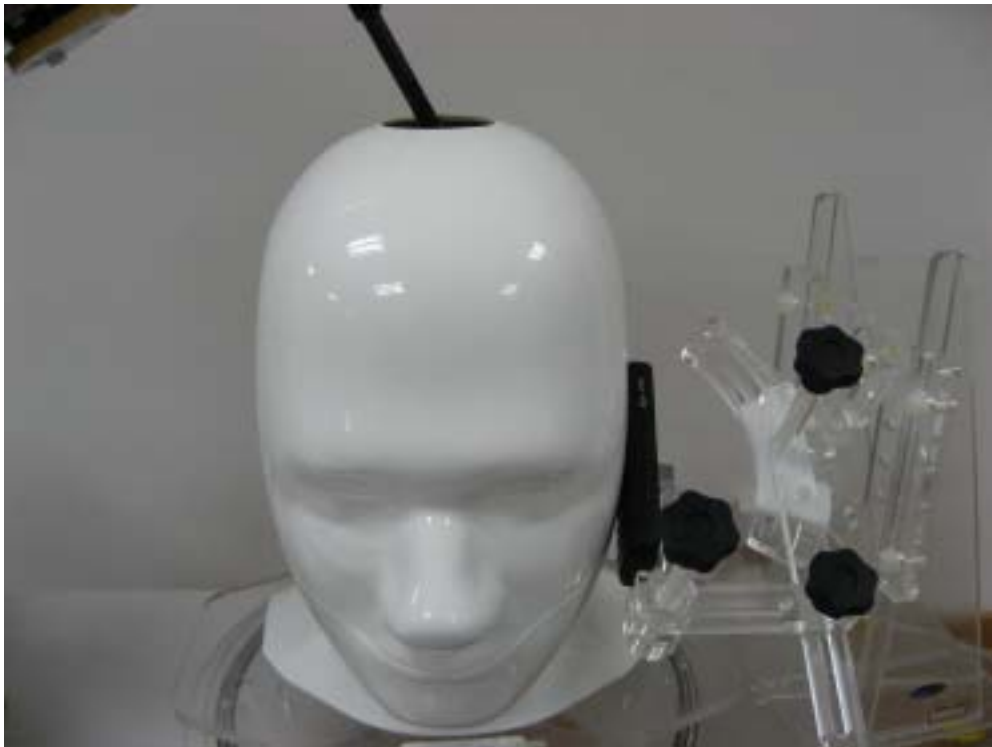
Fig.3 EUT Left Head Touch Cheek Position
