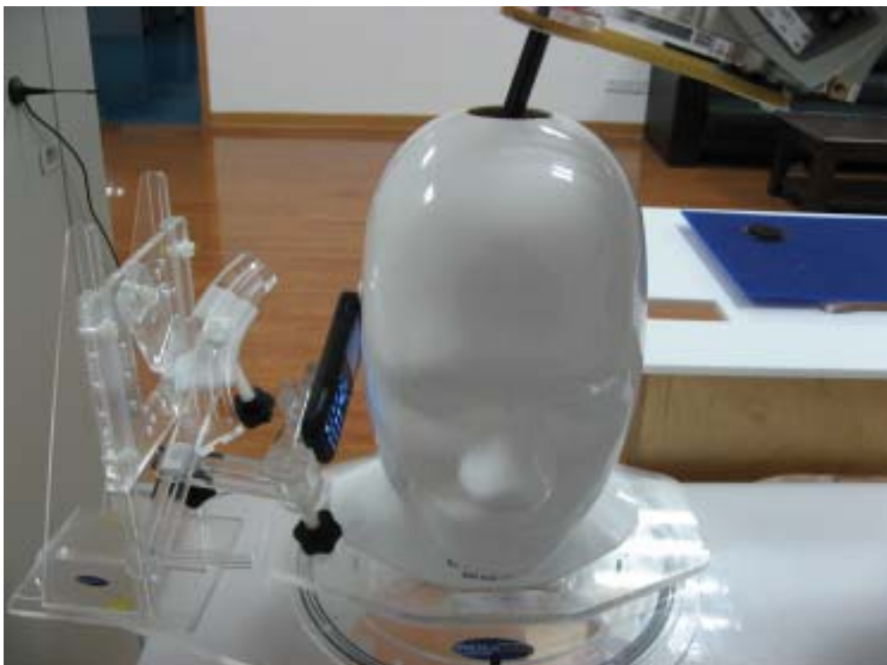
Fig.6 EUT Right Head Tilt15 Position
