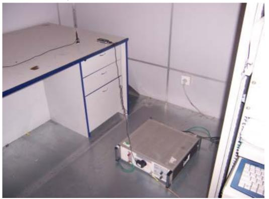
2. Conducted Emission Test, USB Mode
