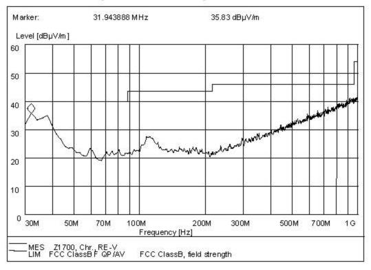
2. Radiation disturbances, maxpeak detector, antenna polarization: Horizontal
