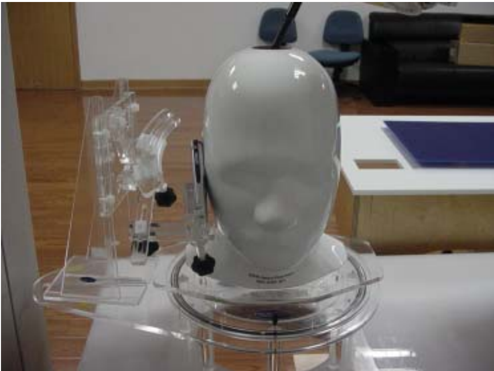
Fig.5 EUT Right Head Touch Cheek Position
