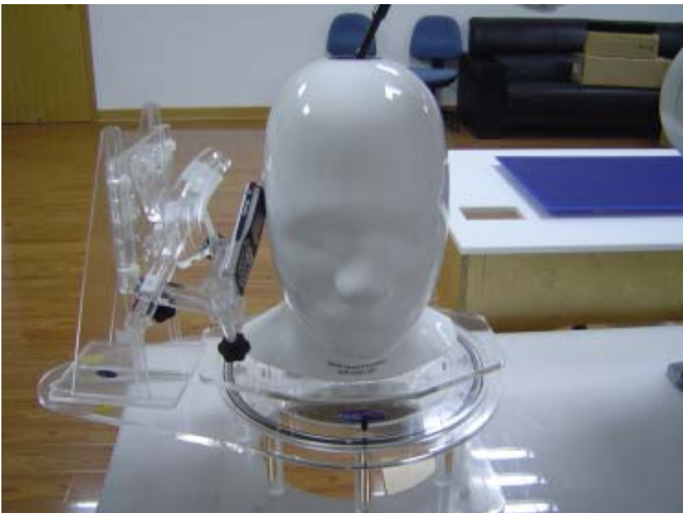
Fig.6 EUT Right Head Tilt15 Position
