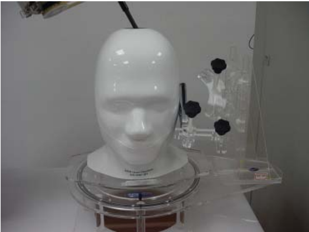
Fig.3 EUT Left Head Touch Cheek Position
