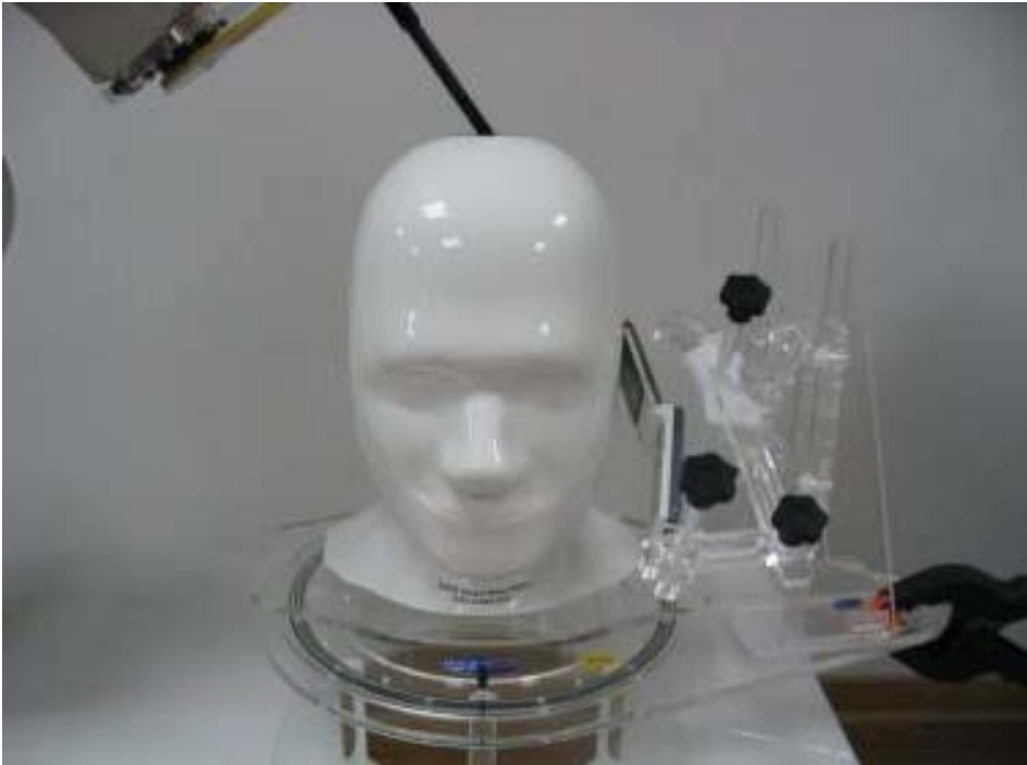
Fig.4 EUT Left Head Tilt15 Position
