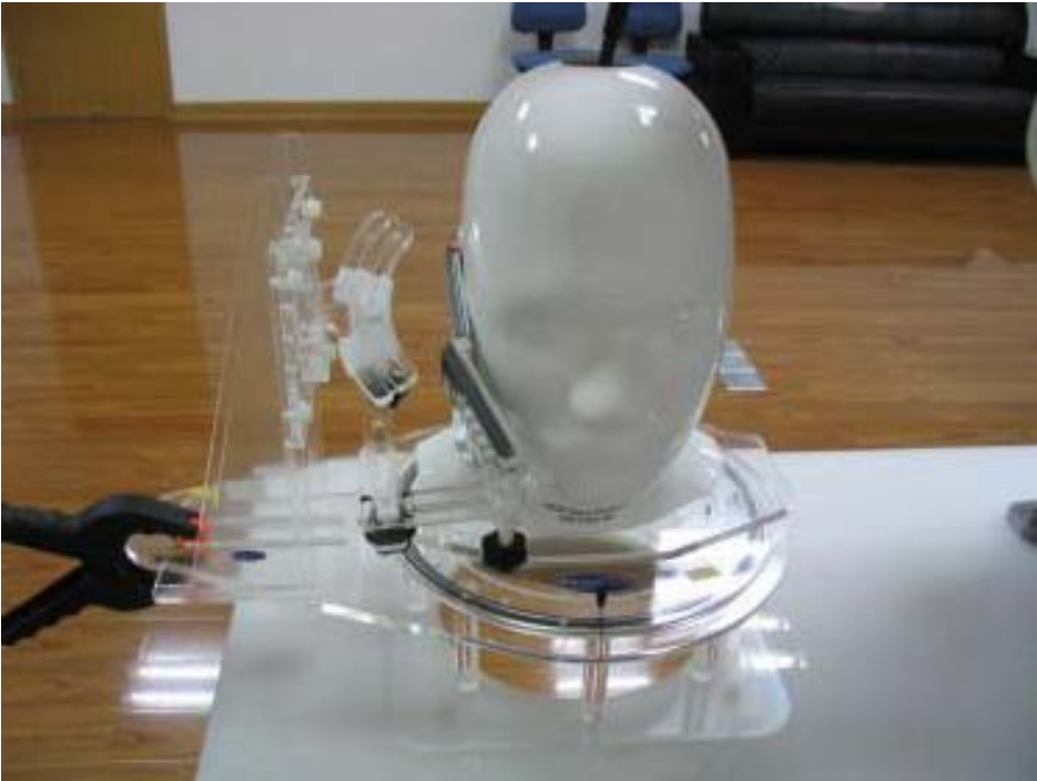
Fig.5 EUT Right Head Touch Cheek Position
