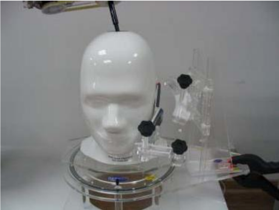
Fig.3 EUT Left Head Touch Cheek Position
