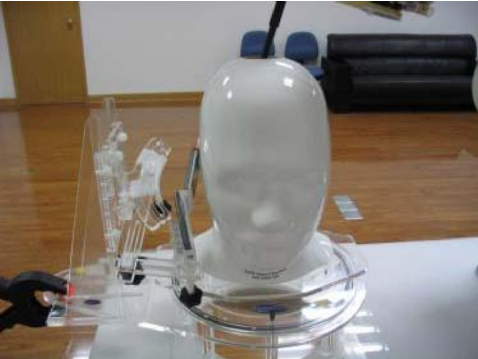
Fig.6 EUT Right Head Tilt15 Position
