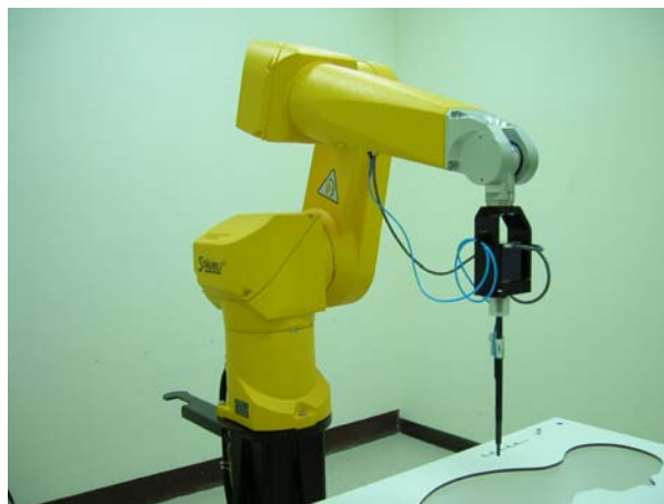
Fig. 5.2 Probe setup on robot
