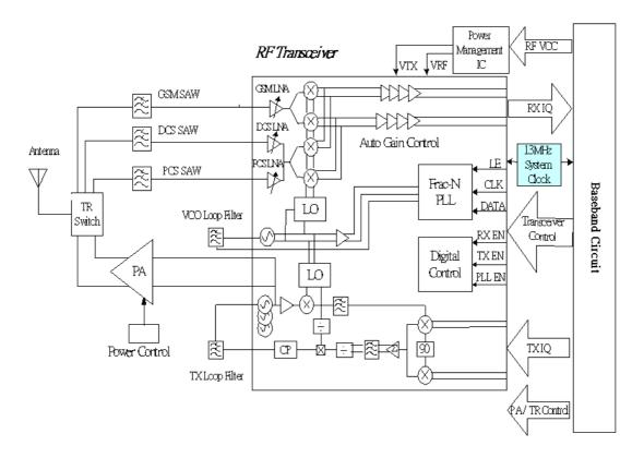
The RF circuits consist of the Skyworks transceiver (CX74063), Power amplifier (CX77315), T/R switch, RF SAW Filter, voltage regulator, TCXO, and some other circuits.
