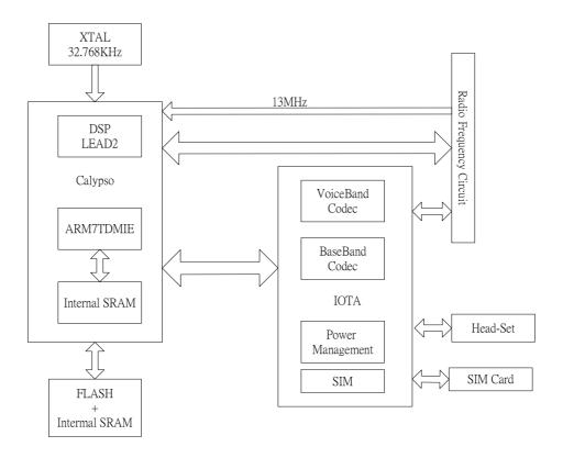
Block Diagram of Base-band Circuit
