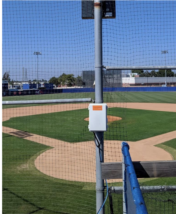
Figure 15 Typical setup of Radar and USB Ext Connection box
