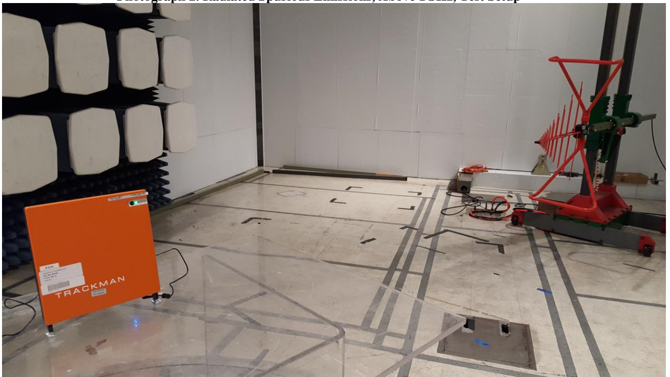
Photograph 3. Radiated Spurious Emissions, Below 1GHz, Test setup
