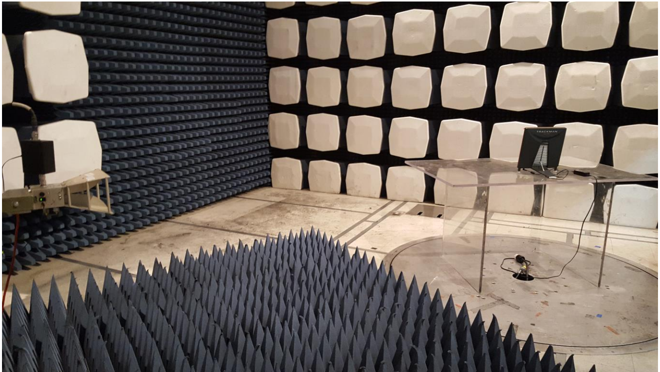
Photograph 2. Radiated Spurious Emissions, Above 1GHz, Test Setup
