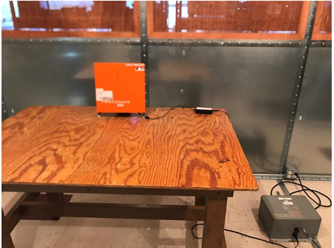
Photograph 1. Conducted Emissions, Test Setup
