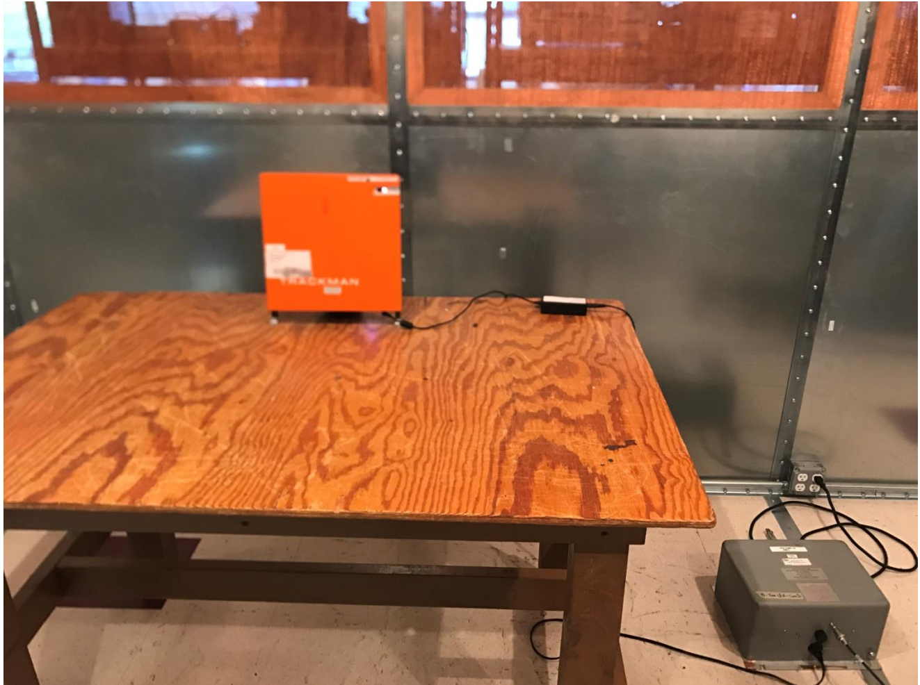
Photograph 3. Conducted Emissions, Test Setup
