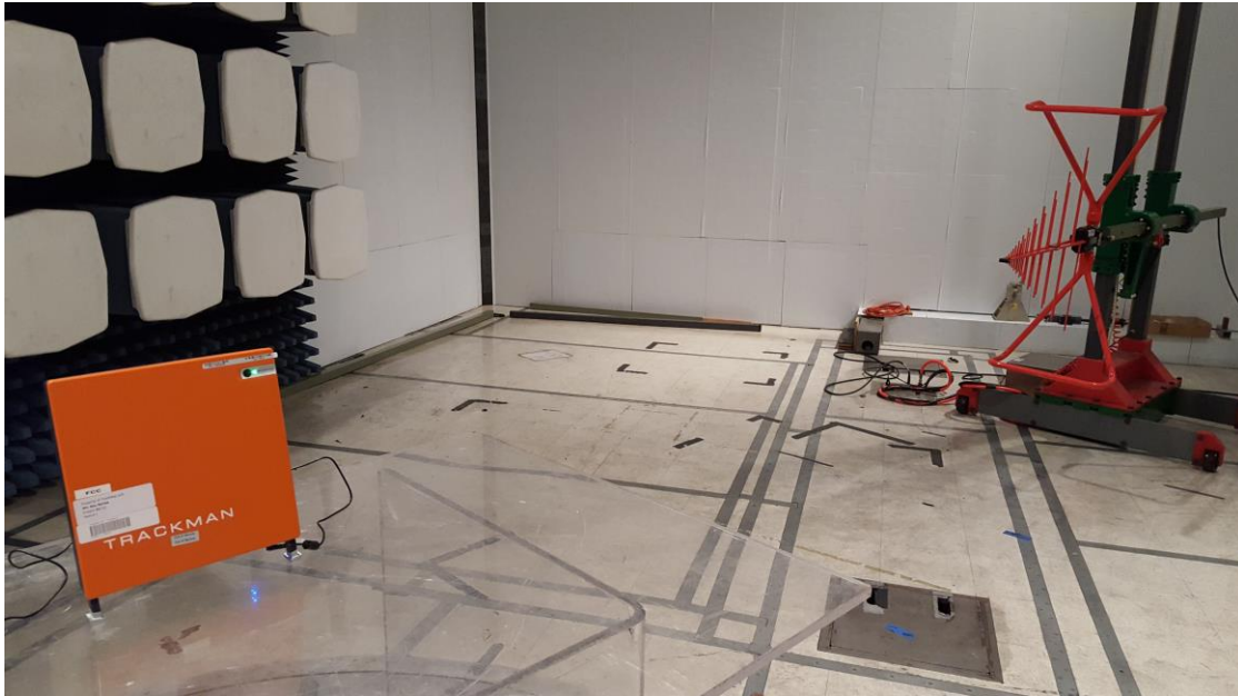
Photograph 1. Undesirable Emissions/Radiated Spurious Emissions, Test Setup, Below 1GHz
