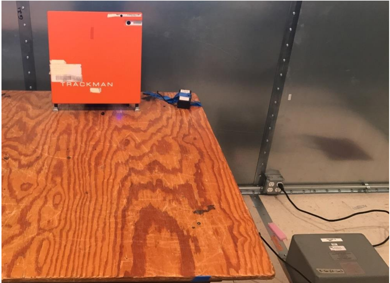
Photograph 3. Conducted Emissions, Test Setup
