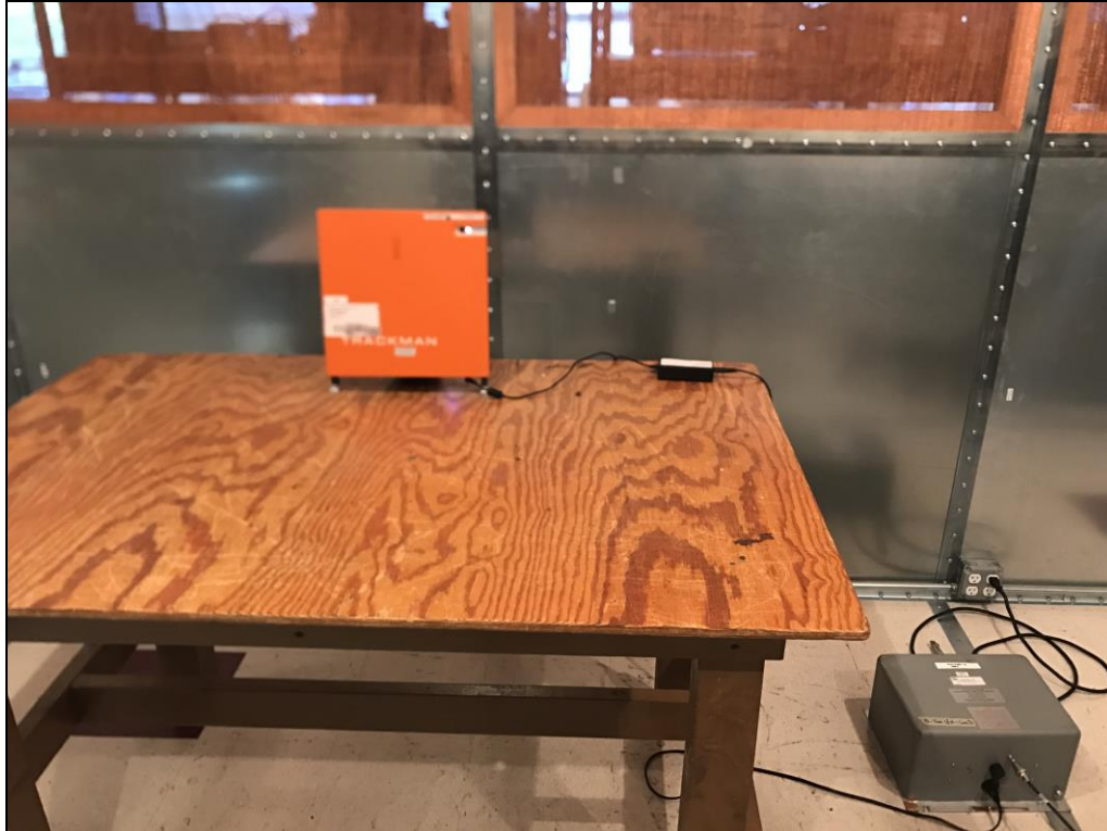
Photograph 2. Conducted Emissions, 15.207(a), Test Setup
