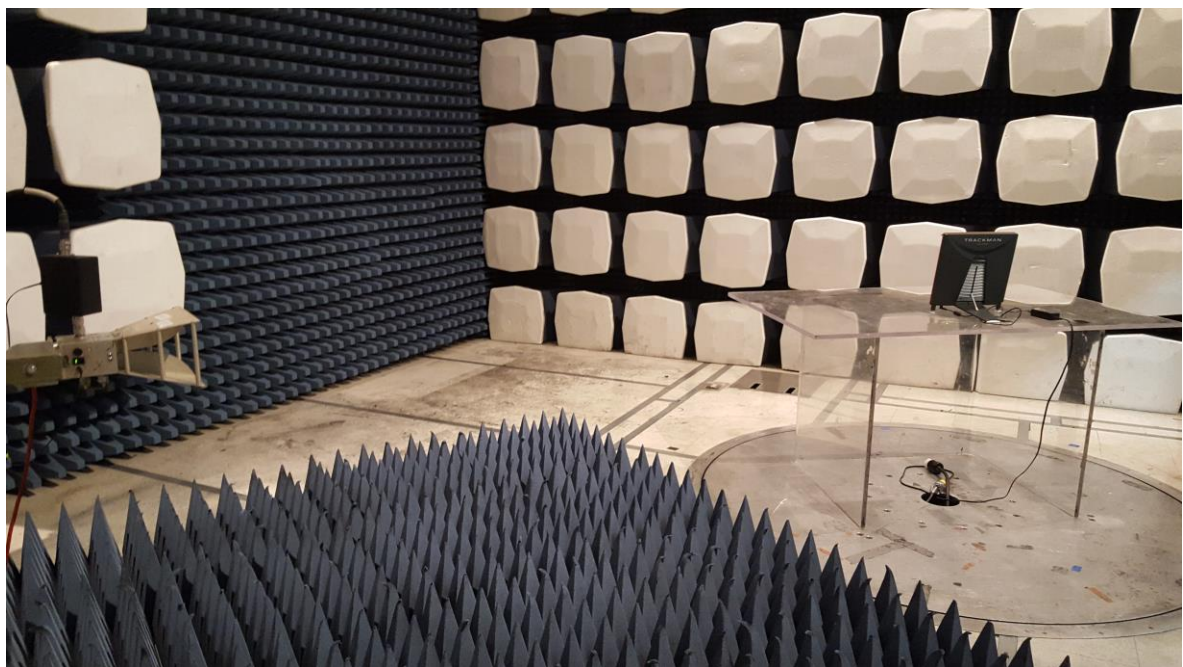
Photograph 4. Radiated Spurious Emissions, Test Setup, Above 1GHz
