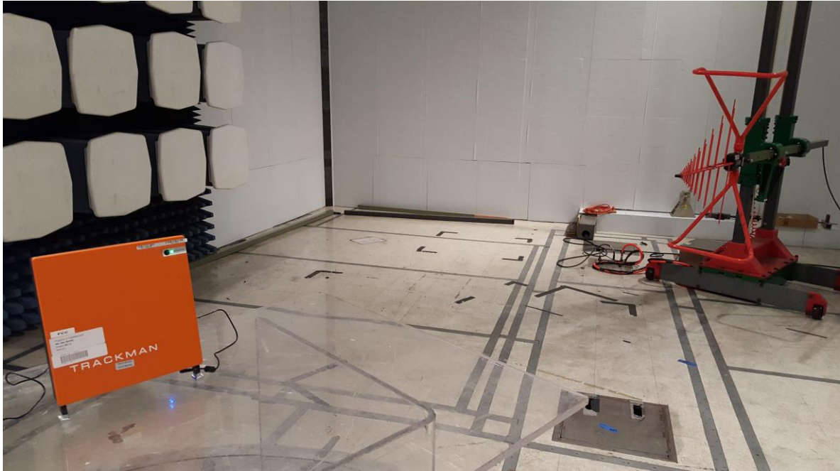
Photograph 3. Radiated Spurious Emissions, Test Setup, Below 1GHz
