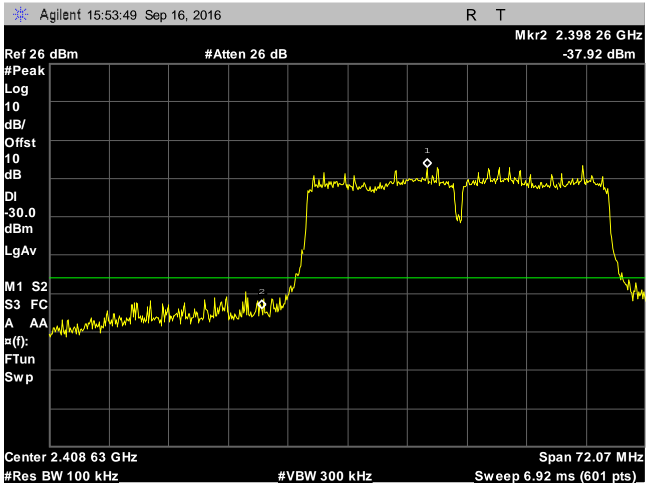
Plot 172. Conducted Band Edge, Ch. 2412, 40MHz, n mode, 30 dBc, Port 1
