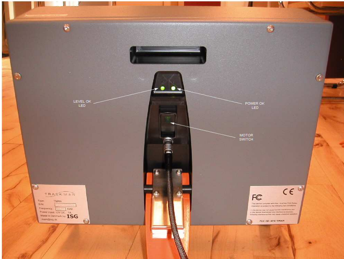
Figure 3: TrackMan™ radar unit, model TMAN back side view
