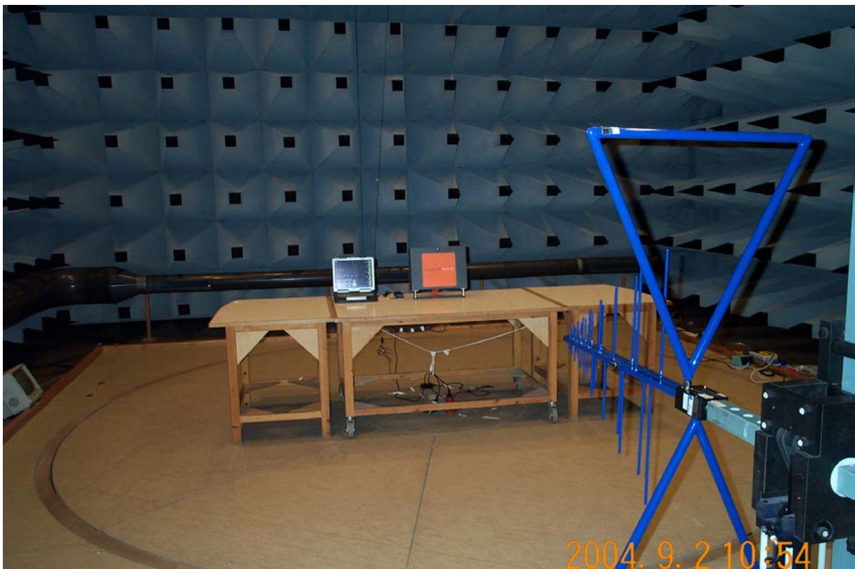
Photo A2.2 Radiated emission 30 - 1000 MHz.
