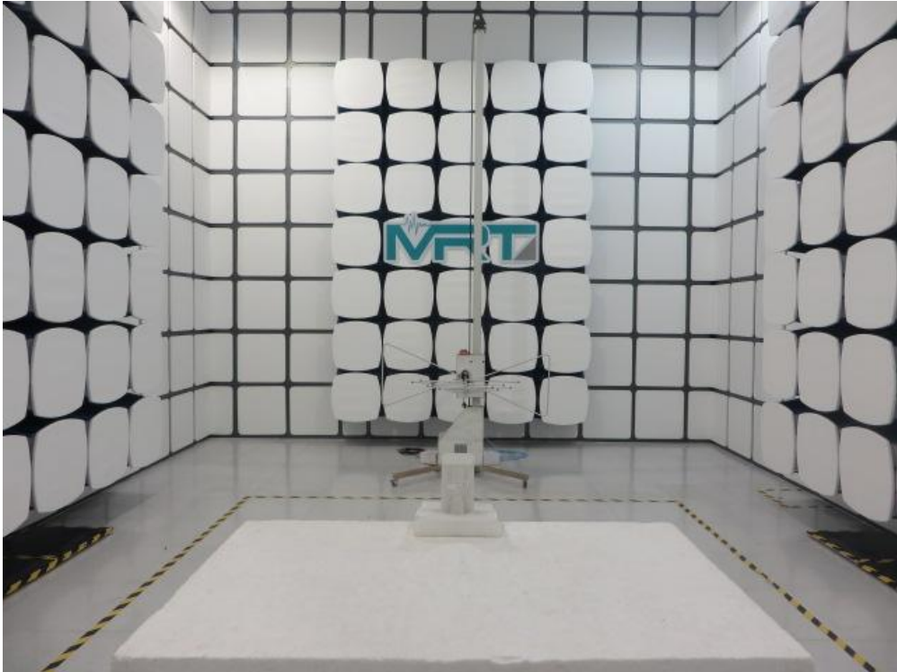
Description: Radiated disturbance Test Setup for 1GHz ~ 18GHz
