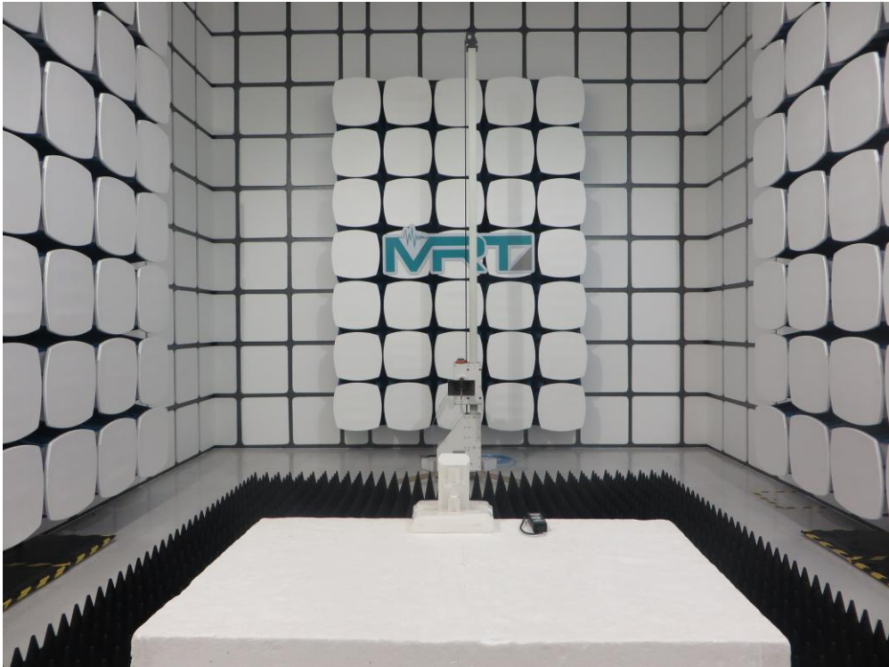
Description: Radiated disturbance Test Setup for 1GHz ~ 18GHz
