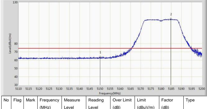
(MHz) Level Level (dBuV/m) (dB) (dB) (dBuV/m) (dBuV) 1 5150.000 63.583 26.131 -10.417 74.000 37.452 PΚ 2 PΚ 5184.745 109.746 72.384 N/A N/A 37.362
