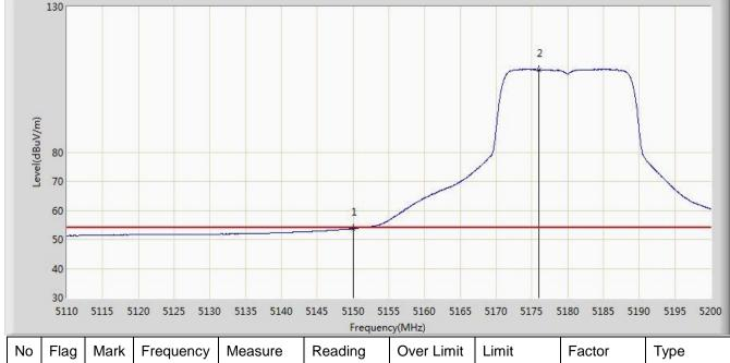
(MHz) (dBuV/m) (dB) Level Level (dB) (dBuV/m) (dBuV) 1 5150.000 53.724 16.272 -0.276 54.000 37.452 ΑV ΑV 2 5176.015 108.356 70.973 N/A N/A 37.383
