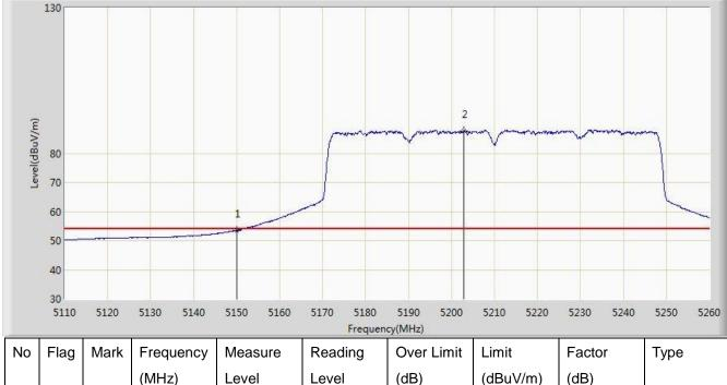
(MHz) (dB) (dBuV/m) (dB) (dBuV/m) (dBuV) 1 5150.000 53.475 16.023 -0.525 54.000 37.452 ΑV 2 ΑV 5202.850 87.643 50.329 N/A N/A 37.314
