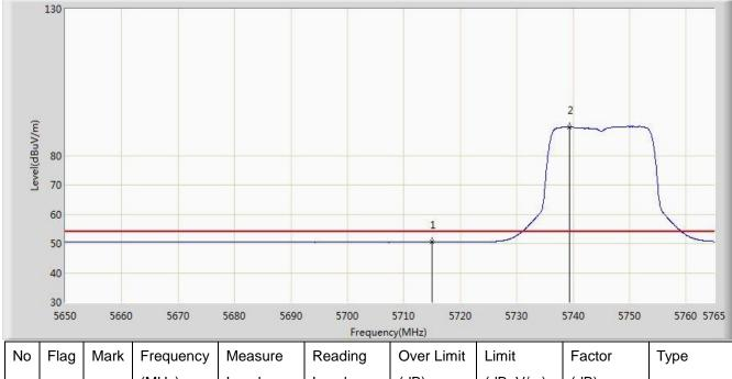
(MHz) Level (dBuV/m) (dB) Level (dB) (dBuV/m) (dBuV) 1 5715.000 50.486 12.537 -3.514 54.000 37.949 ΑV 2 ΑV 5739.355 89.641 51.592 N/A N/A 38.049
