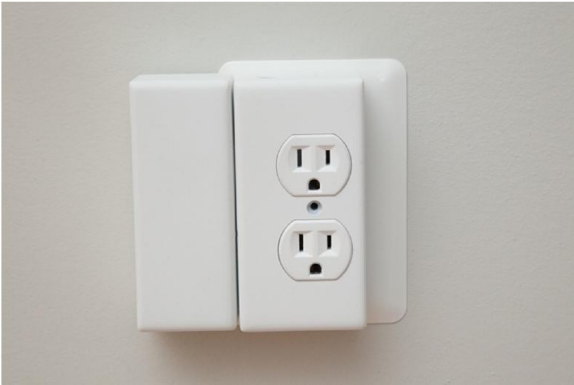
Figure 9: Front view of Location Beacon AC Power (right) with Access Point attached (left)
