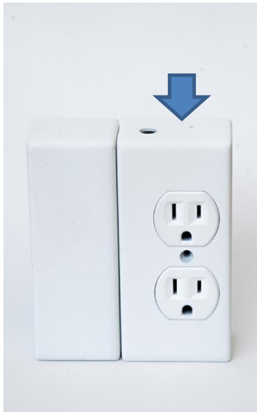
Figure 7: Front view of Location Beacon AC Power (right) with Access Point attached (left)
