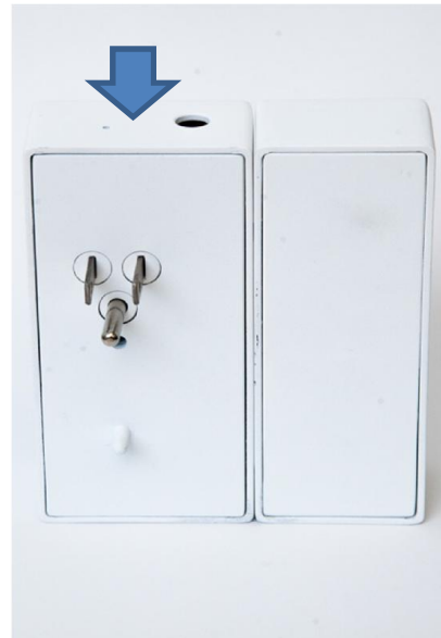
Figure 8: Rear view of Location Beacon AC Power (left) with Access Point attached (right)
