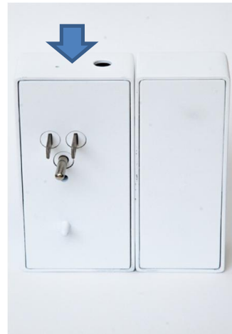
Figure 2: Rear view of Power Cradle AC Power (left) with Access Point attached (right)
