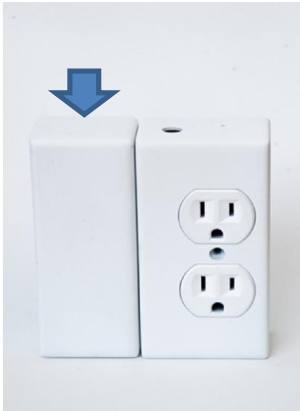
Figure 13: Front view of Access Point (left) attached to Power Cradle AC Power (right)
