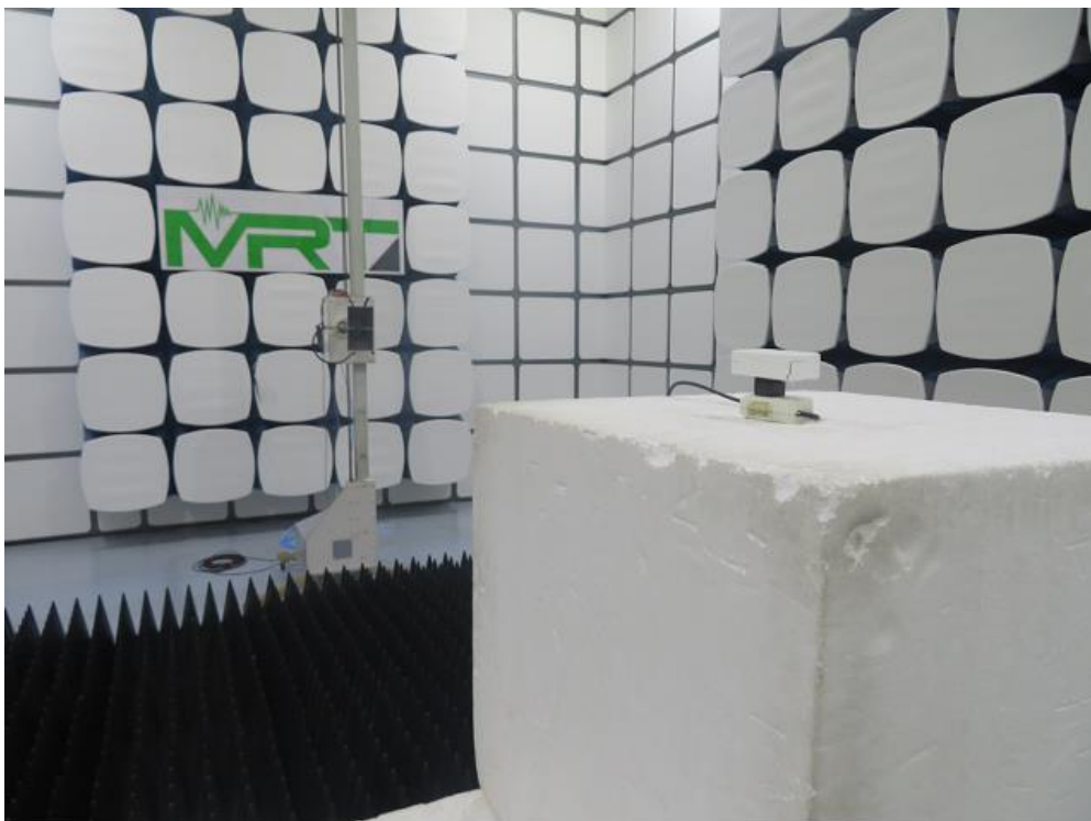
Description: Radiated Spurious Emission Test Setup for 1GHz ~ 18GHz (WF-402B)
