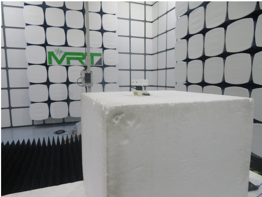
Description: Radiated Spurious Emission Test Setup for 1GHz ~ 18GHz (WF-402CB)
