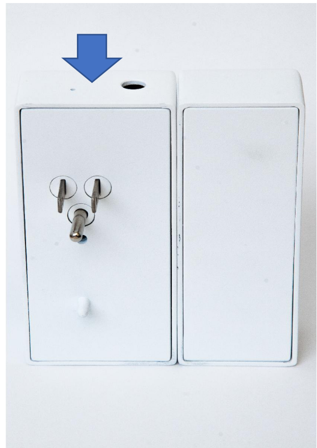
Image 2: Rear view of Power Cradle AC Power (left) with Access Point attached (right)
