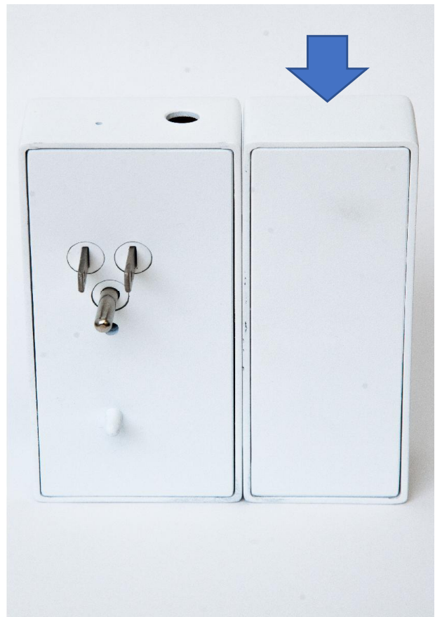
Image 14: Rear view of Access Point (right) attached to Power Cradle AC Power (left)
