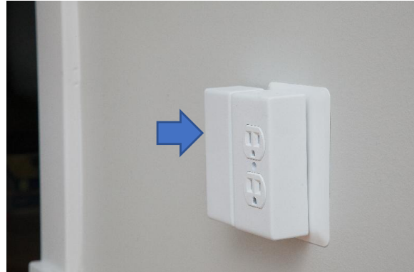
Image 16: Side view of Access Point (left) attached Power Cradle AC Power (right)
