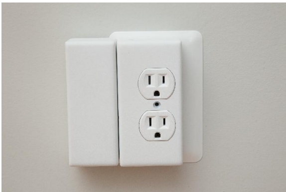
Image 9: Front view of Location Beacon AC Power (right) with Access Point attached (left)
