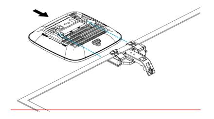
3.4. Go through locking holes by cable\_tie to safely content AP with bracket
