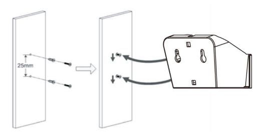
3. Align the securing hookof AP with bracket, and push AP from up to down until it has been locked fully.
