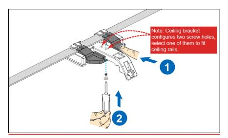
2.3. Align securing hookof AP with bracket (see dotted line), and then push AP close to bracket until AP has been fully Locked
