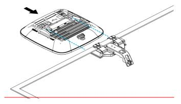
4. Go through locking holes by cable\_tie to safely content AP with bracket
