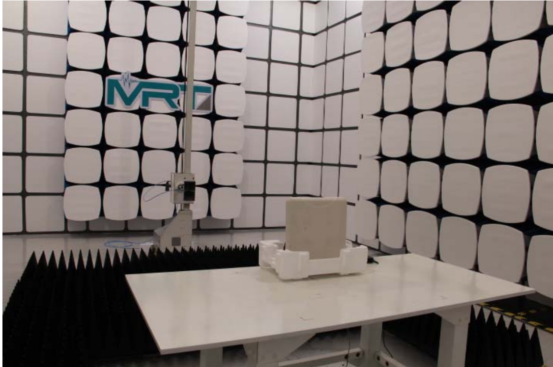
Description: Radiated Emission Test Setup for 18GHz ~ 40GHz
