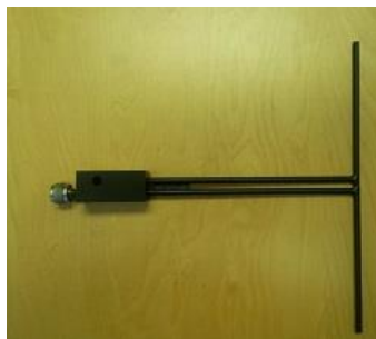
Figure 1 – MVG COMOSAR Validation Dipole
