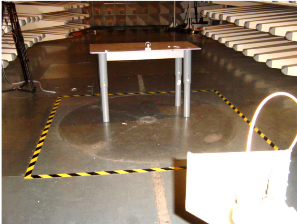
Set-up for Radiation Emission (Transceiver)
