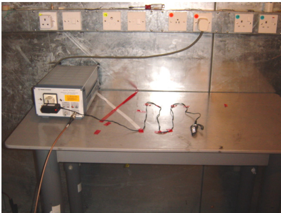
Set-up for Disturbance Voltage on AC mains
