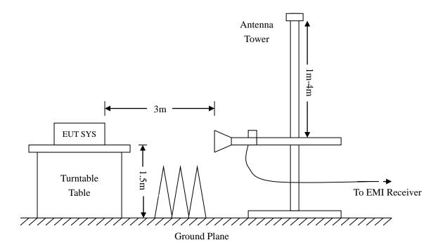
Frequency :9kHz-30MHz Frequency :30MHz-1GHz Frequency :Above 1GHz
