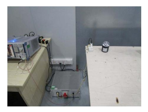
Radiation Emission Test Setup (Below 30MHz)
