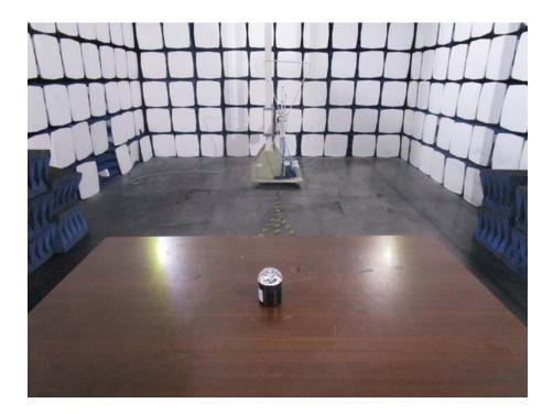
Radiation Emission Test Setup (Above 1GHz)
