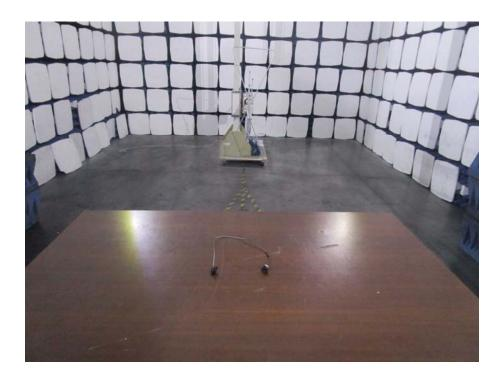
Radiation Emission Test Setup (Above 1GHz)
