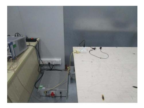
Radiation Emission Test Setup (Below 30MHz)
