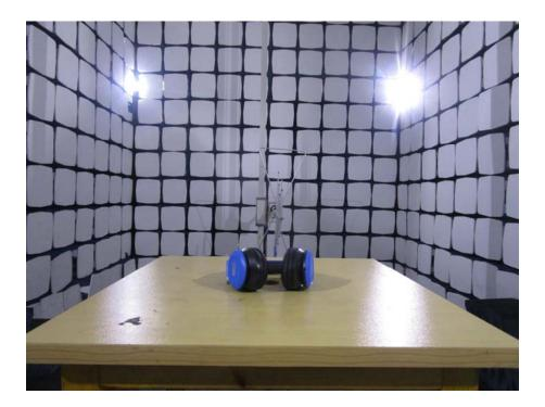
Radiation Emission Test Setup (Above 1GHz)
