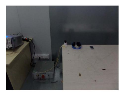
Radiation Emission Test Setup (Below 30MHz)
