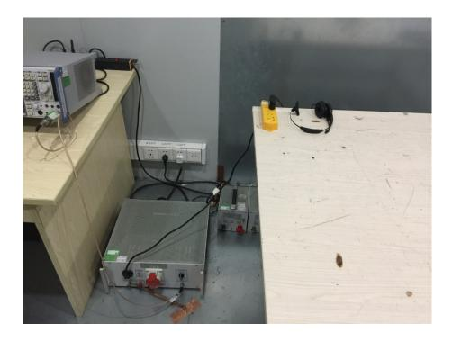
Radiation Emission Test Setup (Below 30MHz)
