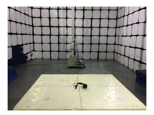
Radiation Emission Test Setup (1GHz to 18GHz)
