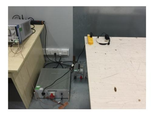
Radiation Emission Test Setup (Below 30MHz)
