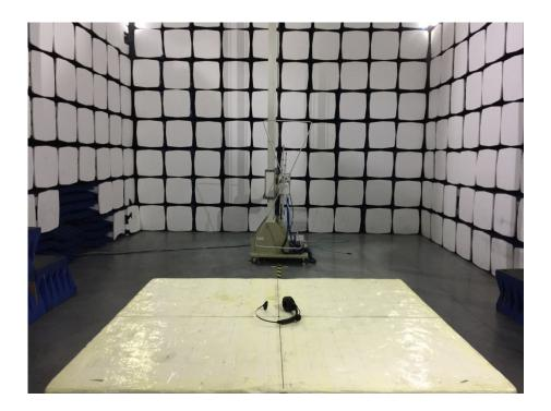
Radiation Emission Test Setup (1GHz to 18GHz)
