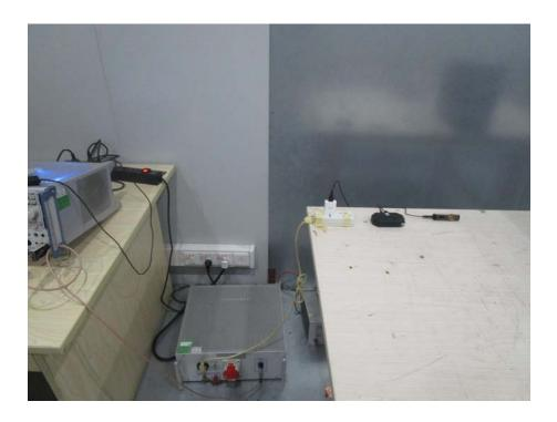
Radiation Emission Test Setup (Below 30MHz)
