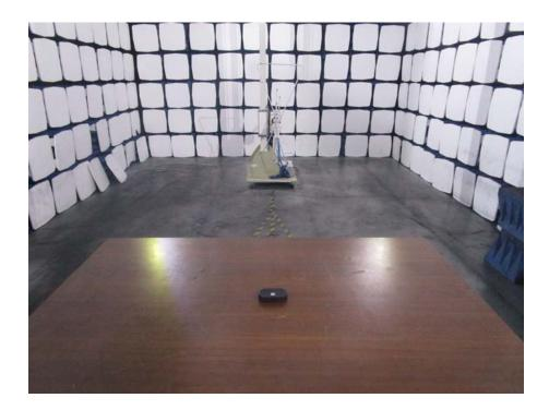
Radiation Emission Test Setup (Above 1GHz)
